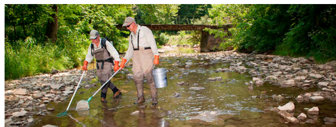
Using electric current to stun fish during a stream survey. Photo credit: U.S. Environmental Protection Agency.
